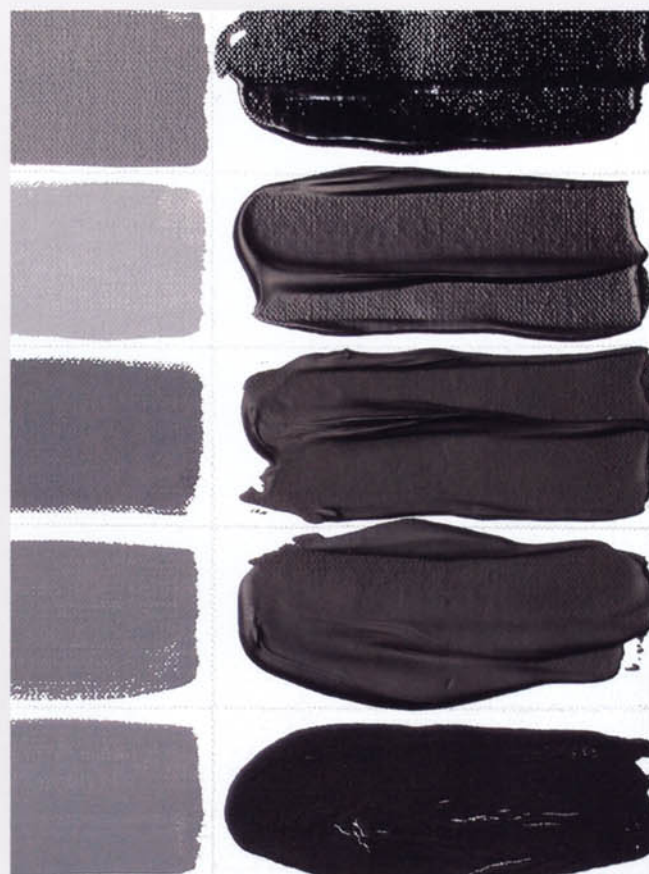
FIGURE 2 Black paints (from top to bottom): Golden Fluid, Guardi, Kreul Solo Goya Acrylic Pastos, Kreul Solo Goya Acrylic Fluid, and Kreul Solo Goya Triton (cracks), with addition of white impasto.
