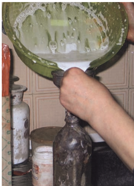
FIGURE 5 (A) Vulcano V7 PVA emulsion mixed with water; (B) paint prepared with V7 and red ochre (both prepared by Sofia Agrela).
