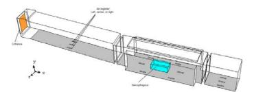
Figure 1b KV1 ventilation grilles locations
