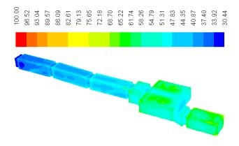
Figure 19 Predicted Contours of relative humidity for KV15 with 8 visitors
