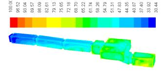
Figure 18 Predicted Contours of relative humidity for KV15 with 26 visitors
