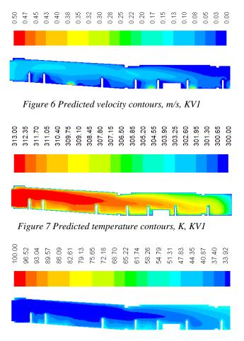
Figure 8 Predicted Relative Humidity, %, KV1
