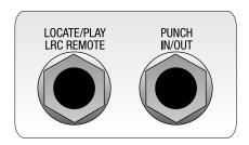
The two footswitch jack functions are designed to be used with any momentary single-pole/single-throw footswitch (either normally open or normally closed). These should be plugged in prior to power-up so that the XT can configure itself for the type of footswitch being used.
