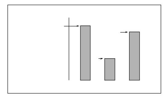
This chart represents three signals which are seen by the DM5. Signal 1 is a legitimate hit from the snare pad. Signal 2 is the Tom 1 pad, but it is not a hit. It is the pad being triggered by stand vibrations from the first snare hit. Signal 3 is a second "real" hit from the snare pad.
