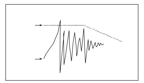
On the other hand, this chart shows the same hit but with the Decay parameter set at a higher value. Notice how the Decay threshold is slightly higher and stays consistent for a longer time before it tapers off. Now only the initial strike of the drum triggers the DM5.
