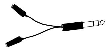
When this setup is used, the footswitch connected to the Tip functions as a Bypass footswitch. The footswitch connected to the Ring functions as a Control footswitch. For more information, see Chapter 2, "Footswitch".
