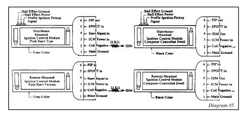
signal travels from pin #4 of the module directly to pin #4 of the ECM.
