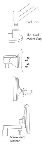
Once the mount is securely fastened, insert the shaft of the arm into the mount cup.
