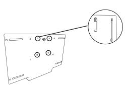
Using the VESA mount positions, attach the Wallmount's wall plate to the PixArm. Mate the monitor to the PixArm by sliding the Wallmount's keyhole slots onto the standoffs. The Display should rest in the padded saddle.
