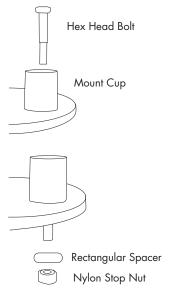
Drill a 3/8" hole into your desk or mounting surface, at least one and one-half to two inches in from edge of the desk.
