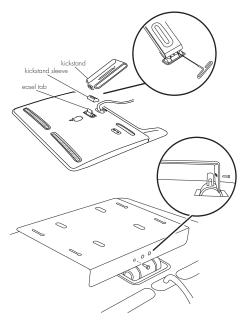
Lay your Cinema Display face down on the non-scratching work surface of your choice. Using the enclosed 2.5mm hex wrench (AKA "Nifty Tool"), remove the three screws to detach the plastic easel from the easel tab. Lift away the kickstand and kickstand sleeve, exposing the easel tab.
