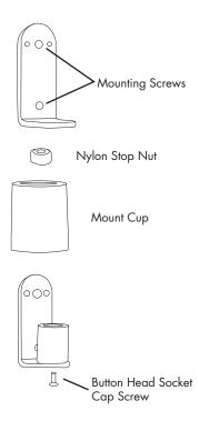
Secure the large L bracket to a stud in your wall using wood screws. Appropriate mounting screws are not provided.
