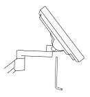
Tilt the monitor so it faces up and locate the set screw under the tilter. Insert the 7/32" allen wrench into the set screw to adjust the tilt friction. To tighten, lightly turn the wrench to the right. To loosen, lightly turn the wrench to the left.
