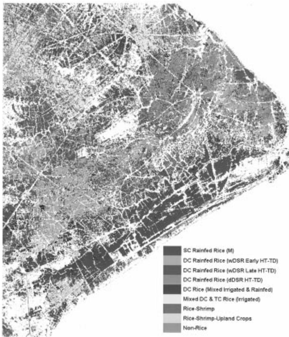
Fig. 2. Thematic classes of rice cropping systems in the Mekong River Delta obtained by hierarchical clustering of the change classes derived from five SAR threshold-change-index maps. See Table IV and text for the rice cropping systems corresponding to each color in the map, and see Fig. 3 for the typical backscattering time series.
