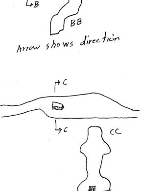
Show cross section and the place from which the cross section was taken. Draw cross sections to scale.
