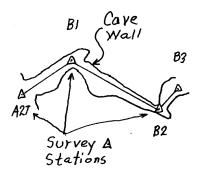
The above sample shows a survey that begins at survey station A27. A27 is a station from an earlier survey and the beginning point for the above sample. The new survey stations are labeled B1, B2, B3, and so on.
