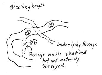
The illustration at the bottom of the page at left shows a passage that passes under the passage being surveyed. Where that passage goes beneath the survey, show the passages walls using a dashed line. Where a connecting passage that is not actually surveyed is sketched in, sketch it using dashed lines.
