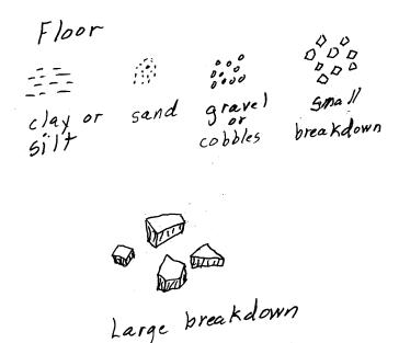
Show floor features as shown above positioning large breakdown blocks to scale. Again, be sure to place notes off to the side of the sketch as to the type of material on the floor.
