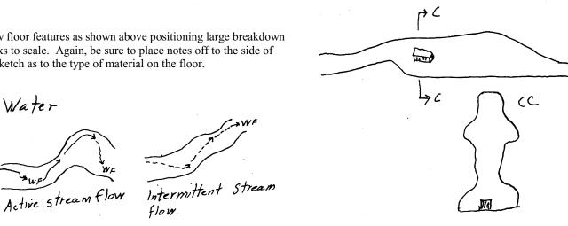
Show active streams as solid line with an arrow indicating the direction of flow. I add the WF to indicate water flow.
