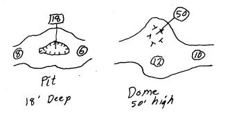
A pit in the floor of the passage is indicted like a contour line on a topo map. The depth of the pit is shown in the box. For the depth of the pit, use the same units that are being used for the survey. If the survey is being done using feet and tenths of a foot, use feet and tenths of a foot. If the survey is being done in meters, give the depth of the pit in meters.
