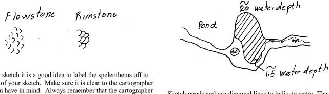
Sketch ponds and use diagonal lines to indicate water. The water depth is shown by putting a wavy line over the number giving the water depth.
