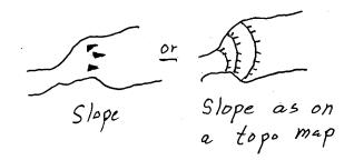
Passage floor slope can be shown using either technique shown above. The technique on the left uses the NSS standard symbol while the one on the right shows the technique that is used on topographical maps. I tend to prefer the technique shown on the right because one can show relative slope by indicating the drop between contour lines – for example 5 feet.
