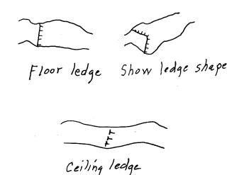
Samples of ledges are shown above. Line shows the direction of the drop of the floor or lowering of the ceiling.
