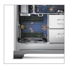
With the removable side panel, DIMM slots are easy to access.
