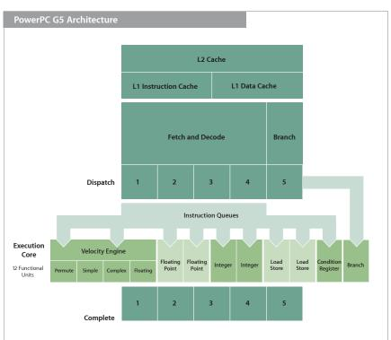
The execution core contains 12 discrete functional units:
