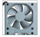
An industry-leading system demands an exceptional enclosure design. The Power Mac G5 features a modern chassis constructed of anodized aluminum. Inside, an efficient cooling system uses low-speed fans for superquiet operation—twice as quiet as a Power Mac G4.
