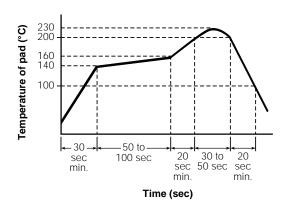
**Recommended Reflow Soldering Profile**
