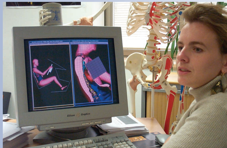
C ESI’s male H-Model (from PAM-Crash) is subjected to a frontal pendulum impact test. The massive pendulum (seen as a bluish square) has compressed the model’s thorax.
