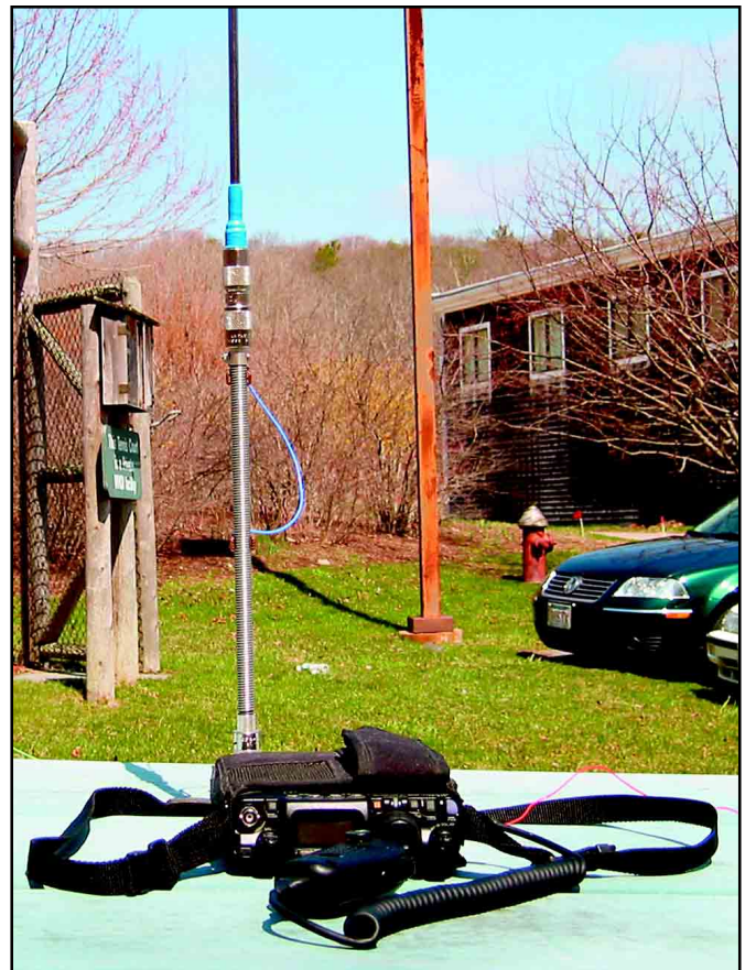
Figure 3—The antenna assembled and mounted on the transceiver. The counterpoise radials can be seen running to the left and right of the transceiver.
