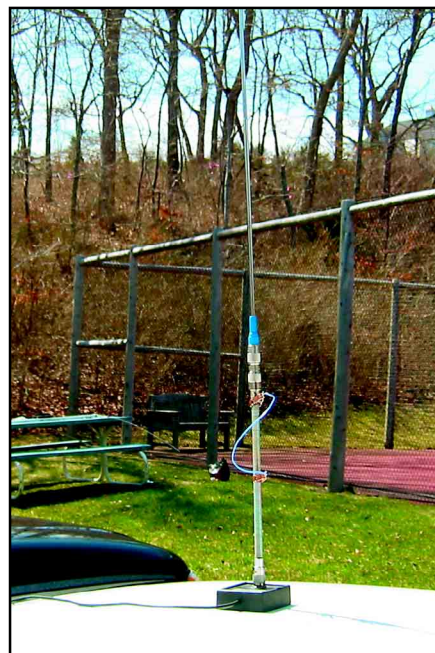
Figure 7—The FARApole used as a stationary mobile antenna with a magnet mount.
