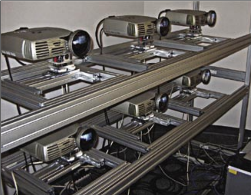
Multiprojector systems, like the one shown here, are supported by PC-based visualization systems, which have been commonly used as the image generator for interactive 3D displays.
