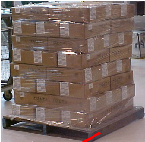
Figure A4: Stack shipping boxes in height of maximum 8 boxes (Typical Example)
