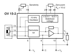
The transmission line between the transducer and the electronic module may measure up to 100 meters. Screened cables should be used to avoid the interference of outside noise.
