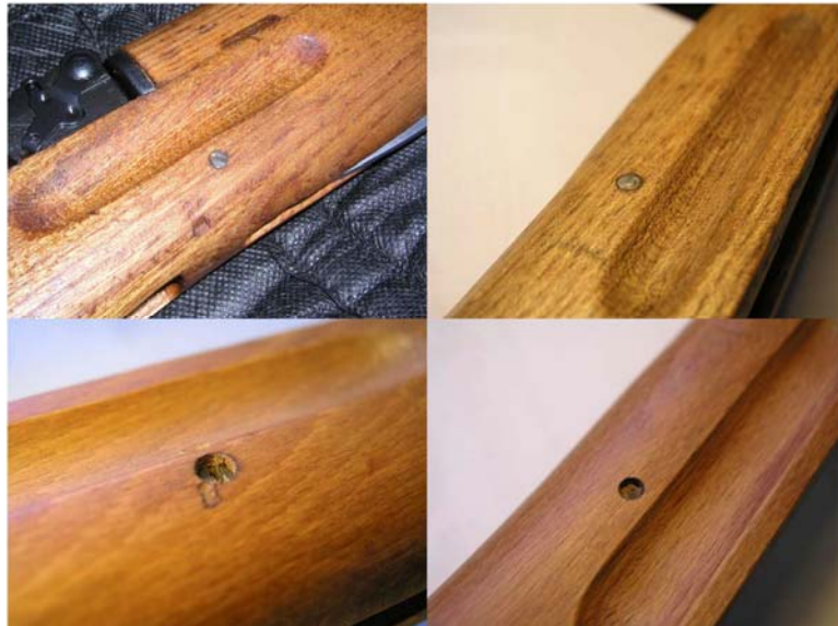
Figure 8. The excessive sanding of the wood around the front stock reinforcing screw. On overhauled rifles, upper two pictures, the stock is sanded all the way to the screw heads. The lower two pictures are taken on the new stock. Screw is recessed in the case of non-overhauled rifle or overhauled rifle with the new stock.
