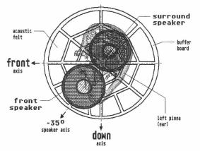
Figure 3: Principle of a circum-aural four channel headphone (type A) for in front localization with a main de-centric "FRONT speaker" placements based on [3]. Furthermore a de-centric speaker to reproduce REAR tone signals in the vertical hearing plain.
