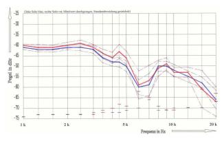
**Figure 5:** Diffus-field transfer function (DFTF) no. 4 of a circum-aural headphone with a centric speaker (lined); the standard deviation (dotted) and the maximum values (dashed); the left channel is colored blue and right is colored red.
