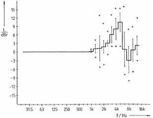
**Figure 2:** Transfer function comparison of coupler and dummy-head-measurements via 20 different headphones (lined), the third octave standard deviation
