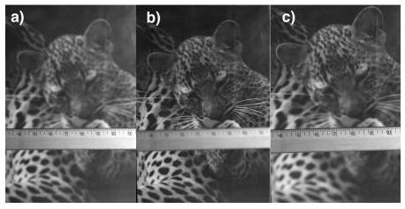
Figure 5: Pictures of a ruler positioned in front of a poster. 5a shows a photo taken with an untilted lens. 5b shows the result of tilting the lens 30° downwards. For Figure 5c the camera back has been extended so as to refocus on the ruler. The image magnification is now 15% larger than before—a result consistent with increasing the focal length of the lens.
