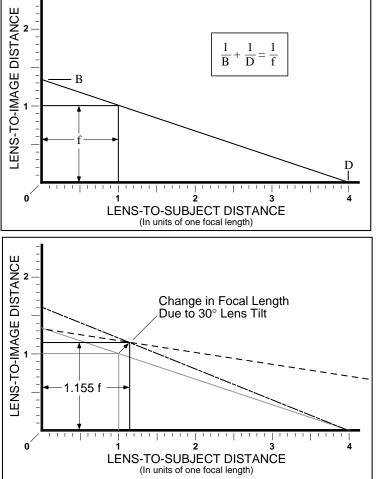
Figure 3: The lens equation relating object distance, image distance and focal length is easily solved with the help of this diagram. Any straight line passing through the top right corner of the square intersects the lens-to-object and lens-to-image scales at points which are valid solutions of the lens equation. An object in front of the lens at distance D will be focused behind the lens at distance B, the back-focus distance.
