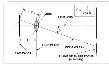
Figure 1: Only along the lens axis is the true focal length of a flat field lens equal to its marked focal length. At other angles, the effective focal length is somewhat longer, as expressed by the formula shown. Examples are given in Table 1.
