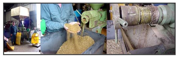
**STEP 2**: Processing the oil. On the Internet, Steven saw many different processors, some very professionally built, others put together with scrap materials. Steven's unit is constructed from new and used water pressure units, steel, recycled plastic drums, bearings, washers, shafting, couplings, fittings and hoses. Steven has made two units, the first (called
