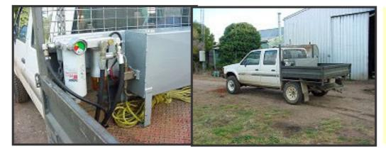
Steven's truck is equipped with a biodiesel kit that allows him to use biodiesel.
