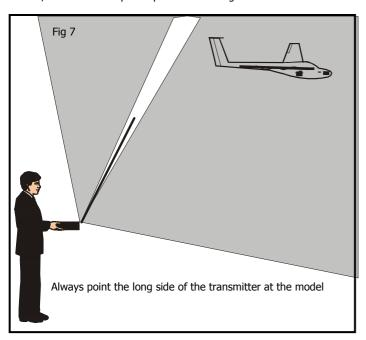
In practice this means that the pilot should always stand with the **long side of the transmitter aerial pointing at the model**, i.e. to achieve optimum reception the aerial should point off at an angle to the model.
