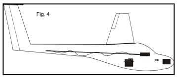
For this reason, deploying the aerial in a gentle curve inside the fuselage is much better than in a dead straight line, as this produces fewer directional effects.
