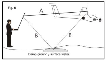
In our experience, based on measurements at a number of sites, the cause is usually wet ground, or even areas of standing water, which can reflect the signal and cause what are know as run time differences (see Fig. 8). The direct reception path "a" is shorter than the reflected
