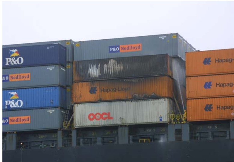
Photo 3. Fire Damaged Containers
