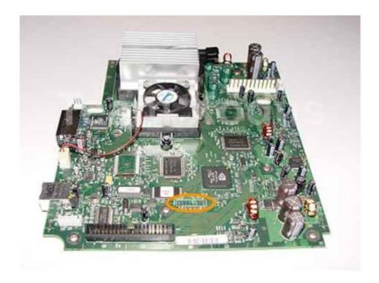
The picture below shows the location of the LPC port on the underside of the motherboard.
