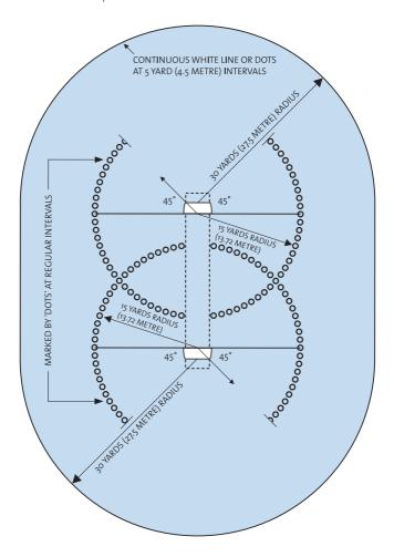
The final mark of the 15 yards radius shall be a line placed at an angle of 45°, measured from the popping crease at a point level with the middle stump
