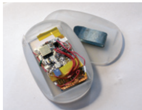
Fried (above, right) works the jammer on an “unsuspecting” cellphone user. The device works by employing a high-frequency oscillator circuit (left) to blanket the immediate area with junk signal.
