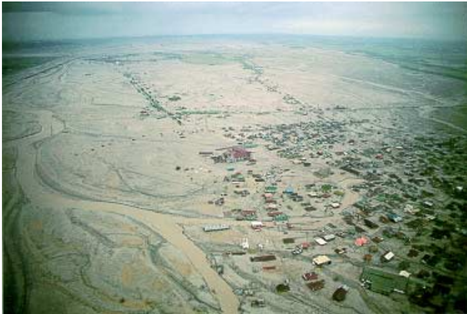
Figure 4: Several cubic kilometers of tephra ejected by Mount Pinatubo in June 1991 was reworked by streams around the mountain during the following years. Above, lahars of Pinatubo ash along the Abacan River buried the town of Bacalor to depths of 15 feet in the town proper, and more than 30 feet in some outlying villages (photo by C.G. Newhall, USGS).
