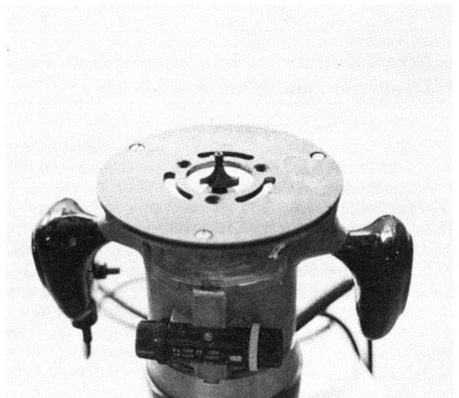
A roundover bit in an electric router is used to radius the edges of homemade plastic deadlights
