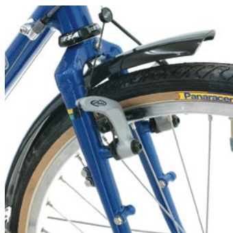
Discreet dynamo mounting boss.
