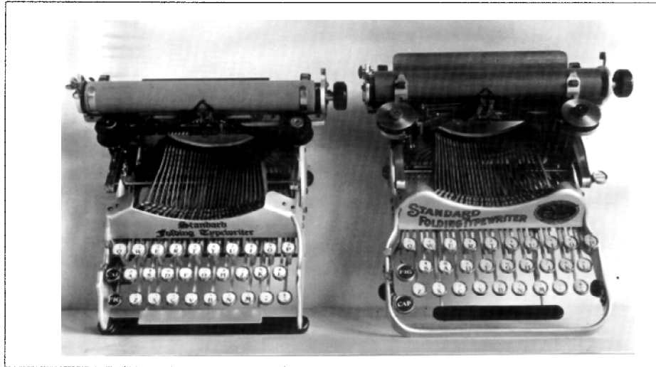
Left: Standard Folding typewriter #2 of 1910. Right: Standard Folding Typewriter #3 c. 1911, a pre-introduction model made before it was named Corona.
