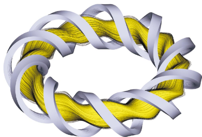
FIG. 5. (Color) The coils and some magnetic-field lines of the Large Helical Device (LHD). The rotational transform in LHD is due to the wobble of the magnetic-field lines produced by the helical coils. A typical plasma has an average major radius of 3.6 m. Figure courtesy of the National Institute for Fusion Science, Japan.
