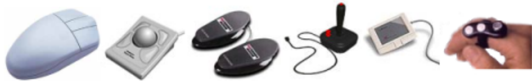
Figure 10.1. A plethora of pointing devices: mouse, trackball, foot-operated mouse, joystick, trackpad, and a finger-mounted pointing device.
