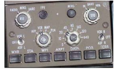
M-Cab HSI Control Panel
