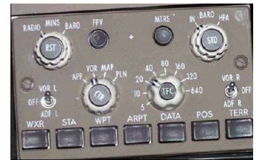
M-Cab HSI Control Panel
