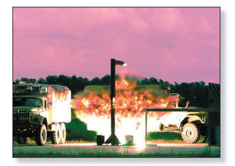
Increased attention to the employment of precision weapons has decreased the occurrence of unintentional collateral damage; however, the development of new munitions to do the same has fallen behind, until now. AFRL's dense inert metal explosive (DIME) successfully demonstrated an effective mechanism to reduce collateral damage, helping the warfighter to prevent the loss of public support and, more importantly, the loss of innocent life.
