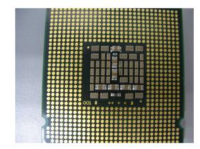
• The Pentium D Processor 960 will change from the 2005 Performance FMB (130W) to the 2005 Mainstream FMB (95W). The processor top marking will be updated as illustrated below.
