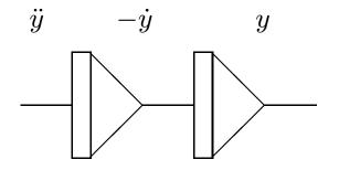
Using a summer with one input the sign of the result can be changed easily:
