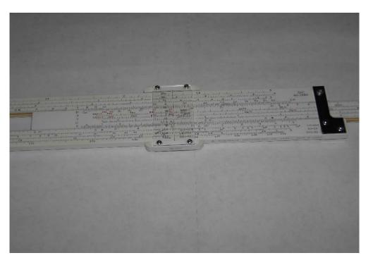
Values are represented by distances which allows easy adding and subtracting of values and thus multiplication and division by using a logarithmic scale.
