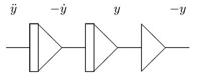
Obviously the left hand side has to equal the right hand side according to the original differential equation, so connecting both sides realizes the equation on the analog computer yielding  $\sin(\omega t)$  as the output of the computer circuit ( $U_0$  denotes the initial condition, usually 1 in this case):
