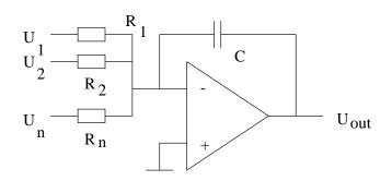
Integration is just as easy as summing – the main difference between a summer and an integrator is that the latter uses a capacitor as its feedback impedance as shown above. The output voltage of the integrator shown above is
