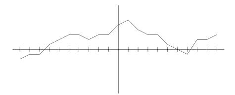
Most implementations have either fixed sampling points (in this case there are normally 21 of these points spaced  $\frac{1}{10}E$  apart where *E* denotes the machine unit (either 10 V or 100 V)) or variable sampling points.
