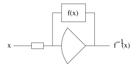
This circuit is normally employed to generate a square root from a square, an exponential function from a logarithmic function, etc.
