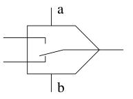
Such a comparator normally has two control inputs a and b. It calculates the sum a + b. If this sum is greater than zero, the relay will be placed in the upper position, otherwise it will be in the lower position.
