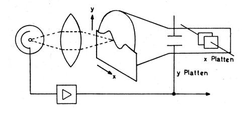
The input to the X-deflection plates determines the position at which the function value has to be determined. The function is implemented as an opaque mask placed in front of the tube screen. A feedback loop will generate an Y-deflection voltage in such a way that the beam will just be on top of the mask, thus following the function.
