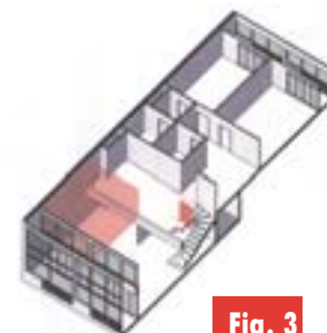
Fig. 3: Perspective cut-away view of double-width apartment. Red hatching indicates space that can be gained by filling in part of the double-height area.
