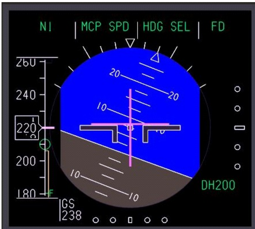
Figure 1.6.2-2 Example EADI Display – In this example, the airplane is pitch is 7.5 degrees above the horizon and the roll angle is 20 degrees to the left, airspeed is 220 knots, ground speed is 238 knots, the autopilot mode is "N1", the pitch mode is "MCP Speed", the roll mode is "heading select", and the autopilot mode is "Flight Director"
