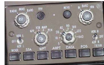
M-Cab HSI Control Panel
