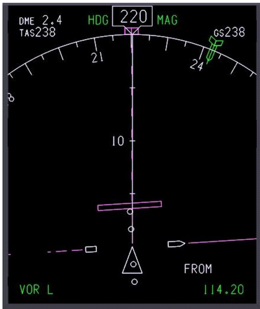
Figure 1.6.2-3 Example EHSI Display – Expanded VOR Mode – Flag notes denote various options
