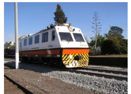
The EM100 train records the alignment of the new track
