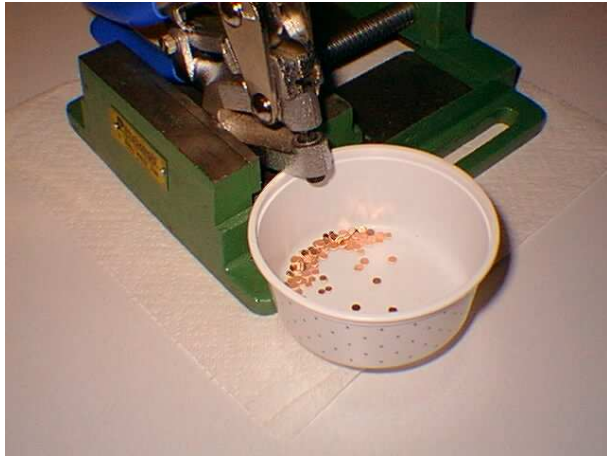
Vise and punch setup for punching pads.
