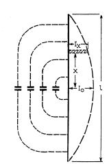
all these l elements of current; in other words, it would be the mean value of  $I_x$  taken over the whole length. Hence the received current at the centre is equal to  $I_{a}$
