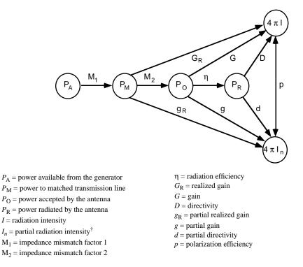
Figure 1—Gain and directivity flow chart
