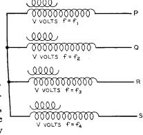
other will be  $\sqrt{2} V$  volts. The remaining two transformers may be left unexcited, or connected in any way which will leave the foregoing arrangement essentially unaltered.
