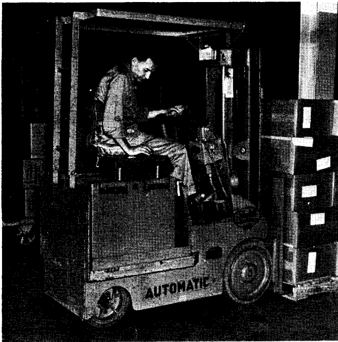
Driver of the electric truck has just deposited a load at the outbound shipping dock. Without dismounting from the truck, and even before the forks leave the pallet, he is able to call the dispatcher for his next assignment
