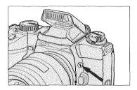
While pressing the flash-control button, press the shutter-release button to take the picture.
