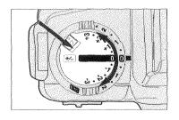
While pressing the lock release, rotate the exposure-compensation dial to set the compensation value. It can be set in increments of 0.5 EV from -3 EV to +3 EV.
