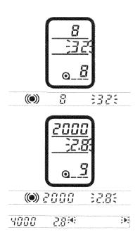
Overexposure; select a faster shutter speed until the display stops blinking.
