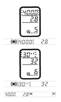
Overexposure; select a smaller aperture (larger number) until the display stops blinking.
