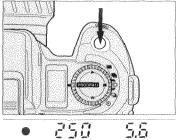
Press the shutter-release button partway down until the focus signal glows.
