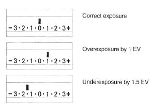
$\bullet$  If your exposure settings exceed the camera's suggested exposure value by more than  $\pm 3$  EV, one of the arrows on the metering index will blink.
