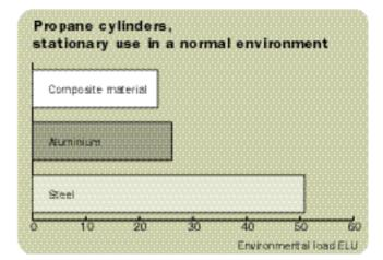
Strong, light products can be made from composite materials. When they are transported, or used in transport applications, the total environmental load is often considerably lower than that of corresponding heavier alternatives.
