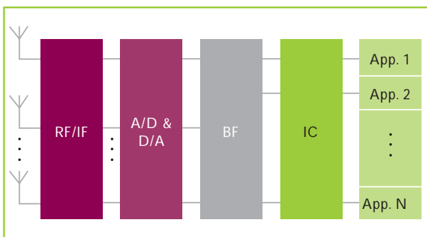
Figure 5-3. Block diagram of the software defined radio demonstrator.
