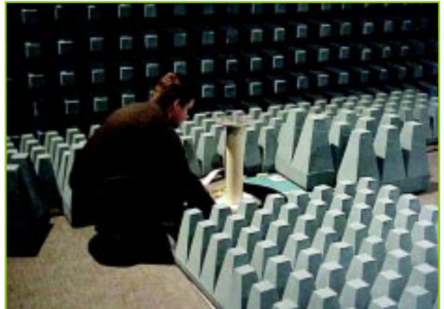
Figure 6-7. Adaptive antenna demonstrator in calibration measurements at the University of Oulu.
