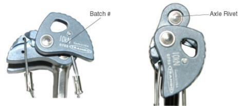
After receiving a defective unit from a climber in the field, in-house inspection and testing has revealed that a small number of our # 1 MaxCams have head axle rivets that do not meet the minimum specified diameter, possibly resulting in failure of the cam assembly. This flaw affects only the red **#1 MaxCam** with **Batch Numbers 0605** and **0705** that were sold in 2005 and 2006. All other cams are unaffected and you can continue to use them with confidence.
