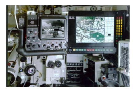
The main elements of the TCCS are the tactical terminal, the command computer, the mission data terminal and the driver's indication unit. The direct link to radio communication equipment warrants high-speed and faultless transmission of tactical situations, commands, messages and alarms.
