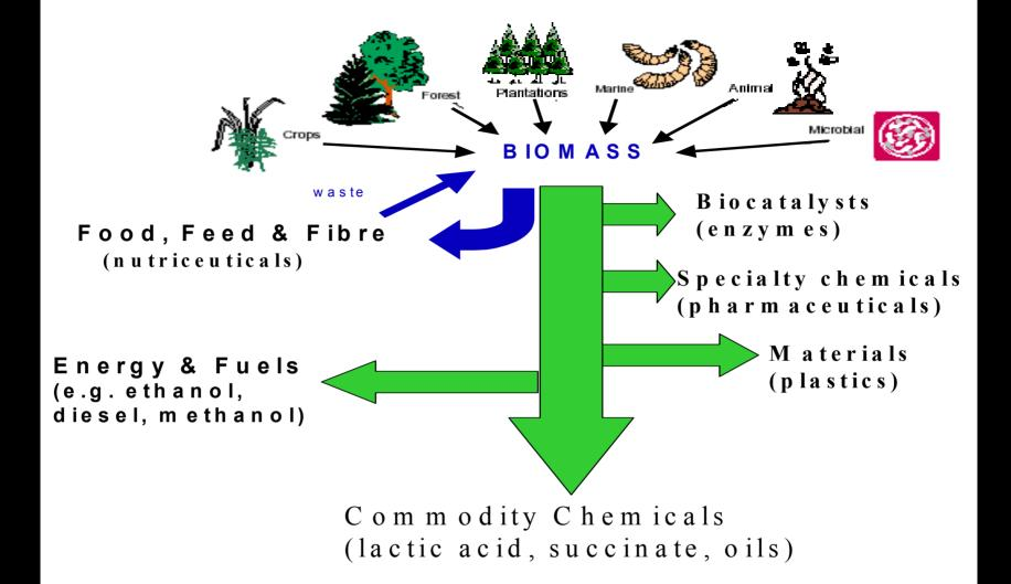
Schematic representation of a bio-refinery
