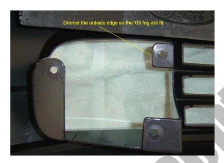
You may need to Dremel part of the mount to make the fog light assembly fit in the hole. Note that I Dremeled part of the mount away for a good fit. This is trial and error but make sure you don't Dremel too much of the mount away. Note that the other two mounting holes are not used.
